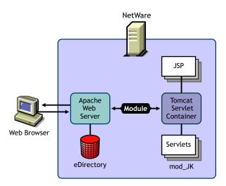
The mod\_jk plug-in opens a socket to an instance of Tomcat and communicates with it using the AJP 13 protocol. Tomcat processes the HTTP request and then returns an HTTP response, which is sent back through the same socket connection to Apache. Apache then serves the response up to the client that requested it.
