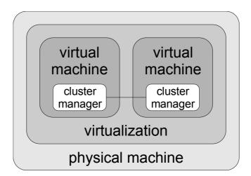
This setup does not protect against hardware failures. So the physical machine itself is a SPOF (single point of failure). Other advantages normally offered by
