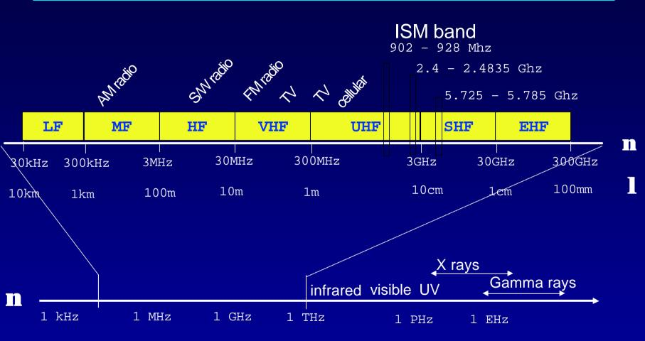
Propagation characteristics are different in each frequency band
